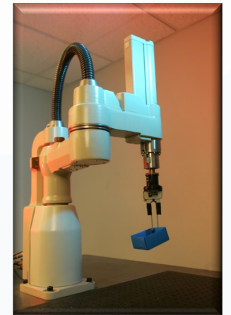
SCARA Robot Source: TEMPUS IV Project: 158644 – JPCR Development of Regional Interdisciplinary Mechatronic Studies - DRIMS
